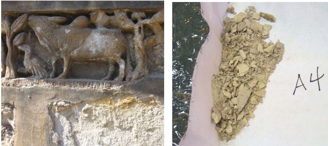
Figure 13: Location of Sample A4 (left) from the exterior of the Bhandarkhal Tank pavilion and detail of sample (right).
