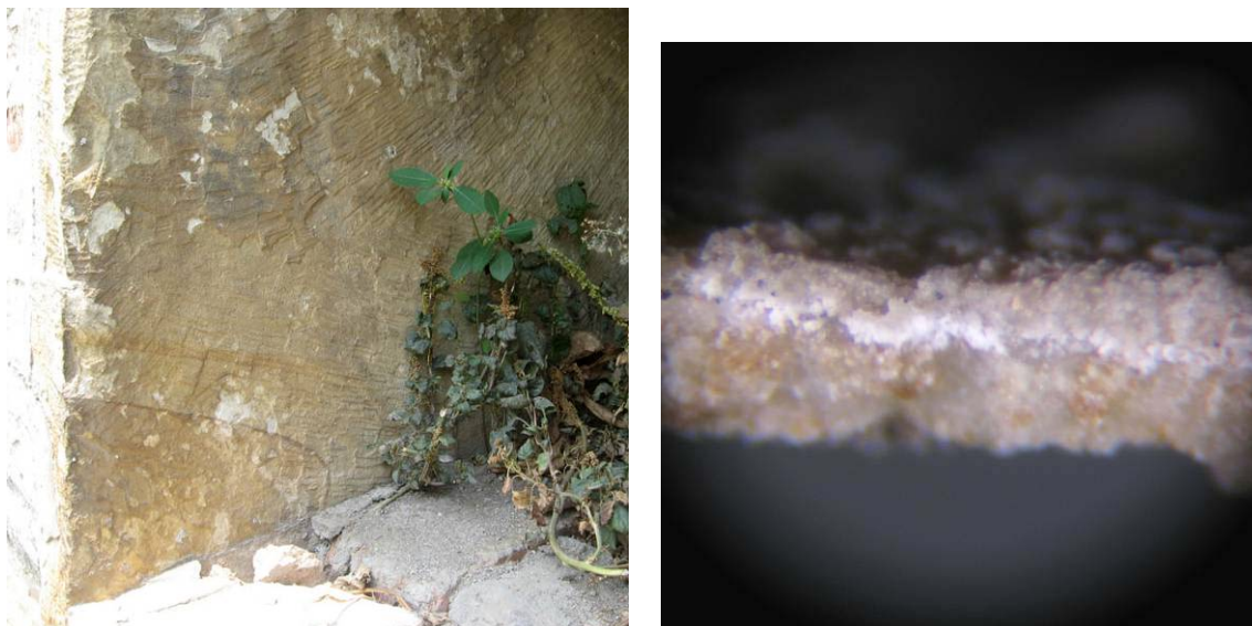
Figure 18: Location of Sample S2 (left) at the Bhandarkhal Tank and detail of sample (right).
