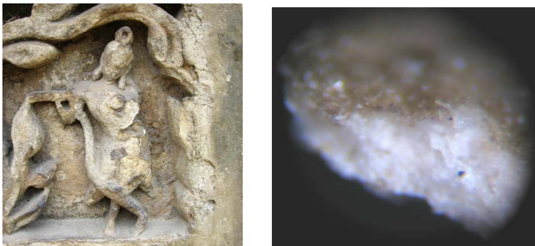
Figure 16: Location of Sample C1 (left) at the Bhandarkhal Tank and detail of sample with visible coating (right)
