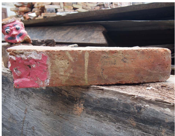
Side view The individual pieces measure approximately: l=48 cm, w=10 cm, h=11 cm
